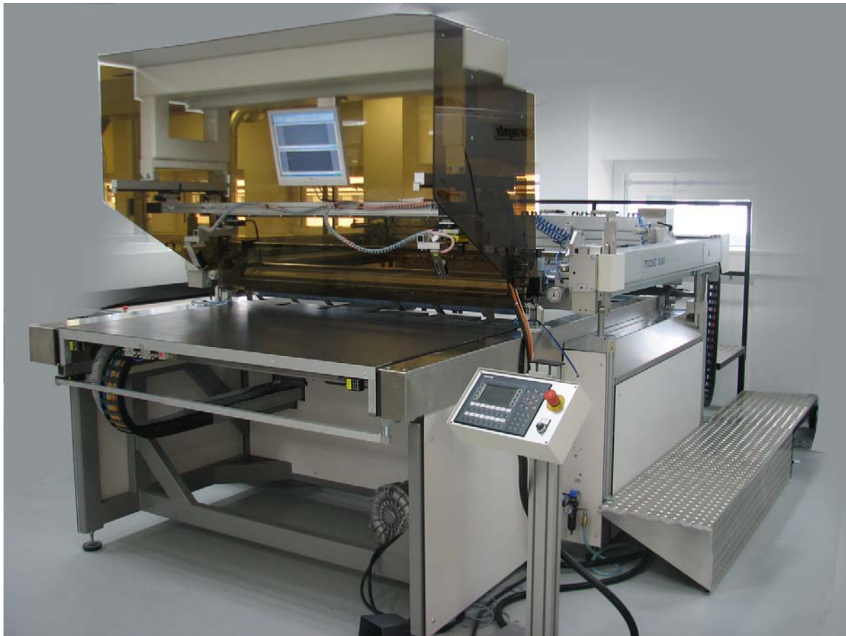
Pic. 1. The screen printing systems THIEME 1000 and THIEME 3000 with automatic print stock positioning were especially designed print table, positional deviations of 0.1 mm can be automatically recognised and corrected within one second.
