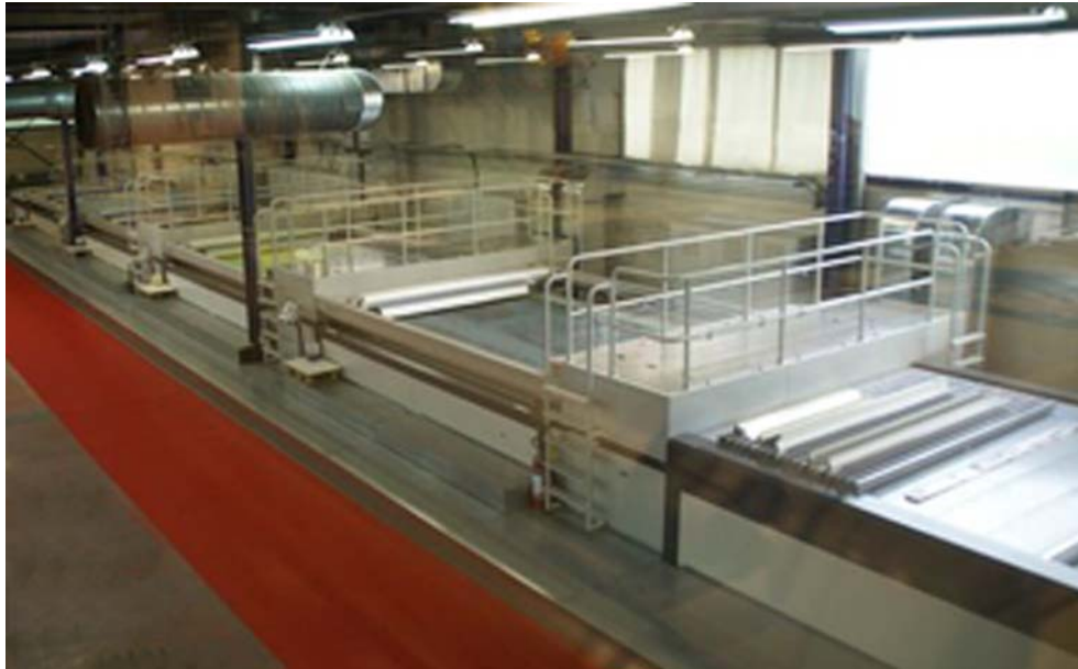
Pic. 1. The new machine THIEME 5000 XXL with short squeegee, long squeegee stroke and the dryer modules designed as UV-bridge system.
