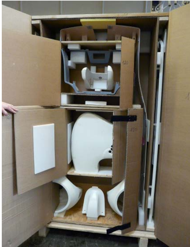
Fig. 2: The new transport packaging, designed according to the poka-yoke principle, prevents random errors, missing parts and transport damages. Every part has its own established place.
