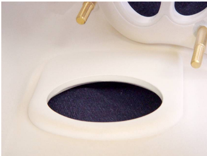
Fig. 4: The complex composition of the housing was enabled by means of variable insulation thickness. To immobilize the housing parts and to assemble the electronics, it makes use of domes, snaps, groove/tongue connections, and inserted nuts.
