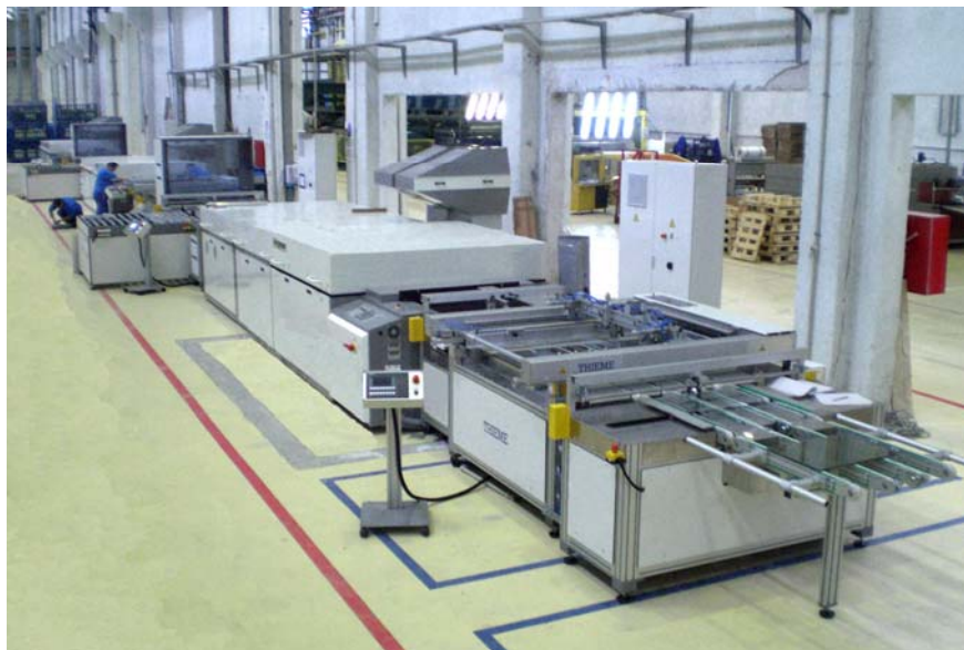
Fig. 2: The three screenprinting stations are integrated into a 45 metre long inline production line at the Targovishte site.
